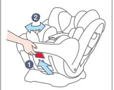
2. Rotate the shell until the white arrow is above the blue arrow.
